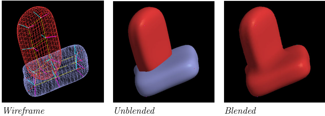
Figure 2.2: An m-rep figure and subfigure blended in Pablo using an implicit surface.
