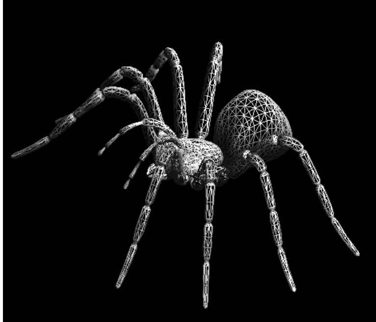
Figure 5.13: The big_spider.ply model from the Computer Graphics Group at the University of Virginia. This model has 9286 triangular faces meshing 4670 vertices.
